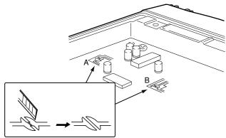
**NOTE:** Be sure to re-solder above print patterns, when you remove the scrambler unit. Otherwise no TX modulation or AF output is available.
